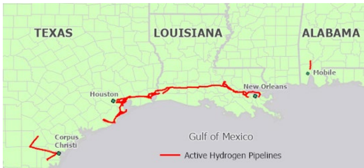
Hydrogen pipelines on the Gulf Coast | Congressional Research Service
